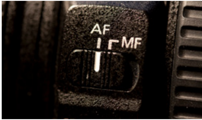
The Auto-Focus / Manual Focus switch. Get used to quickly switching back and forth.
